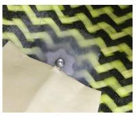
Apply Masking tape over the whole area to enable a smooth and relatively flat blended in surface – if the rivet sticks through the tape, that is ok. You want to be sure that the Star Nut is completely covered so it stays in place when the hole is either chased, or drilled and tapped.
