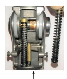
Remove spring assembly from spring seat
