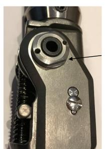
Slighty tighten the Axis Nut.
