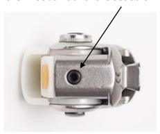
With 4mm hex wrench, turn screw: Clockwise = increase friction Anti-clockwise = reduce friction
